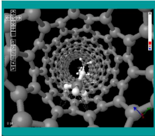
*Figure 1. An all atom molecular dynamics simulation of motion of methane molecules moving through a carbon nanotube [6].*
